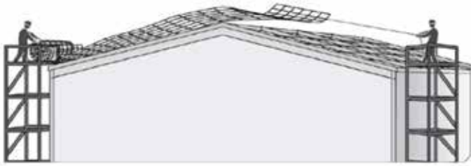
FIG. 2 Crosswire or transverse wire should face up and longitudinal wire should face down. Wire shall be pulled taut allowing for natural sag only.
