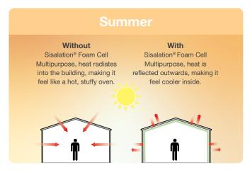
In summer, **Sisalation® Foam Cell Multipurpose** helps keep the heat out. Metal roofs can exceed 80°C causing heat to radiate into uninsulated buildings. Foam Cell Multipurpose greatly reduces this radiation and helps make the building feel much cooler compared to an uninsulated building.
