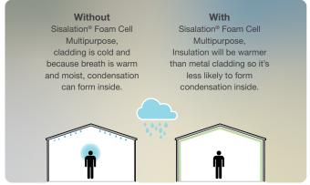
In winter, cold, uninsulated walls quickly remove any heat generated in a building. Sisalation® Foam Cell Multipurpose will reduce this heat transfer and help make the building feel warmer. It will also reduce the risk of condensation by providing an insulating layer between potentially warm, moist air and the cold wall.
