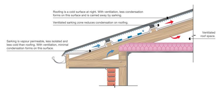
In the unlikelihood of condensation occurring beneath the metal roof cladding, this solution:
