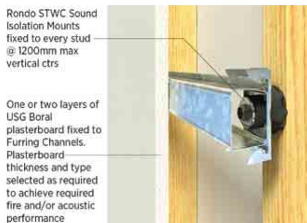
Figure H4: Furred Lining With Sound Isolation Mounts
