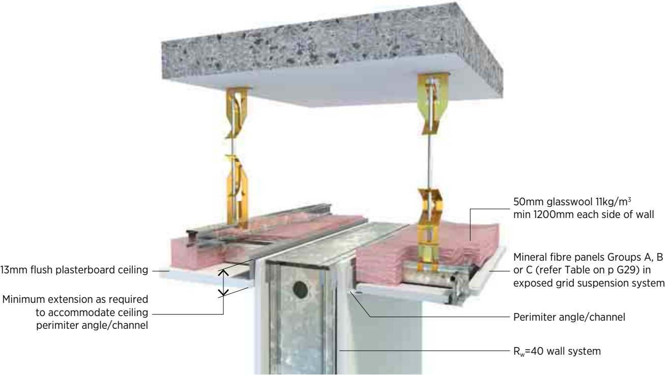
Figure G14: Ceiling configuration to maintain an R w =40 wall acoustic rating (System OP.5 shown)
