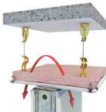
Figure A4: Sound Transfer Over Partition
